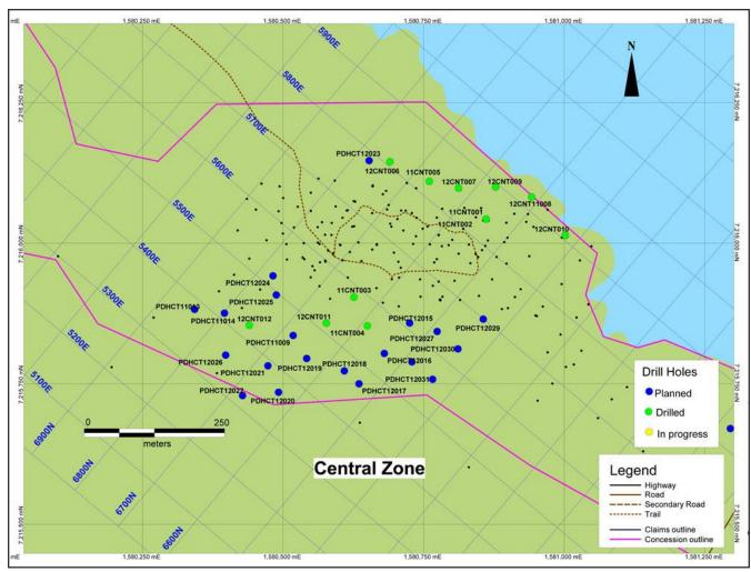
Figure 10.1 Plan View of Drill Collars – Central Zone (Map Credit Orex, 2012)
